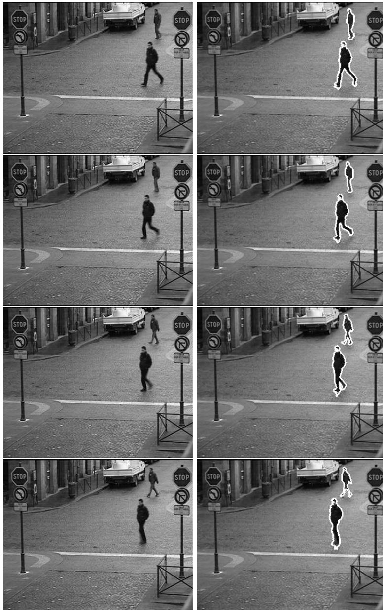
Figure 5.5: Four images of the street sequence. Original images on the left. Detected regions are outlined in white on the right. NFAs are about 10^{-80} on the pedestrian closer to the camera and about 10^{-18} for the pedestrian in the background
