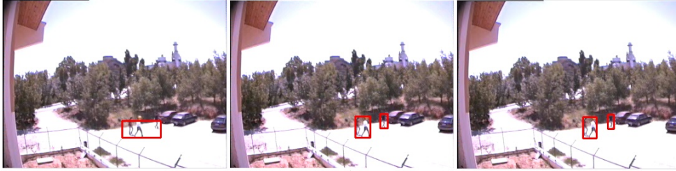
Figure 2.4: Detection results for subband domain(left), VSAM(middle) and GMM based methods in a parking lot sequence recorded in the day-time
